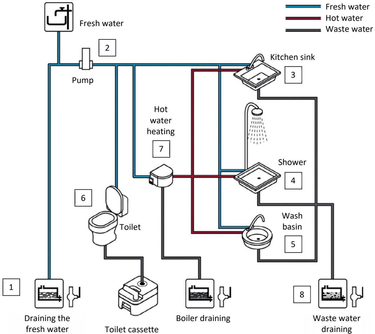
The fresh water system consists of the fresh water tank (1), the fresh water pump (2), the outlet points (kitchen sink (3), shower (4), wash basin (5), toilet (6)), the boiler for the heating (7) providing the hot water for the outlet points, and the waste water tank (8) where the used water is collected.
