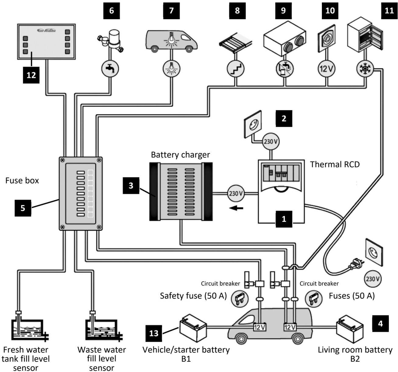
The electrical system consists of a 230 V circuit and a 12 V circuit.
