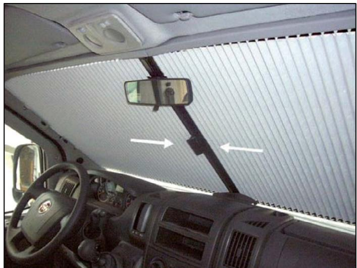
**Closing the side window blinds:** Release the strip from its lock position and carefully pull it to the opposite side.
