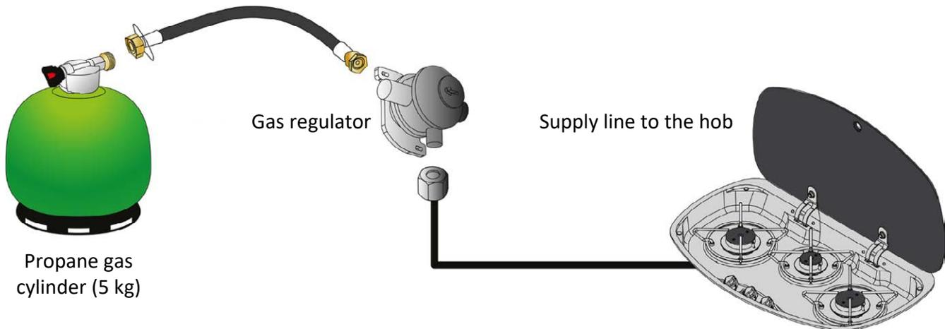
The gas system comprises the gas cylinder with an integrated safety valve (not included), the permanently installed gas regulator and the consuming point – the gas hob.
