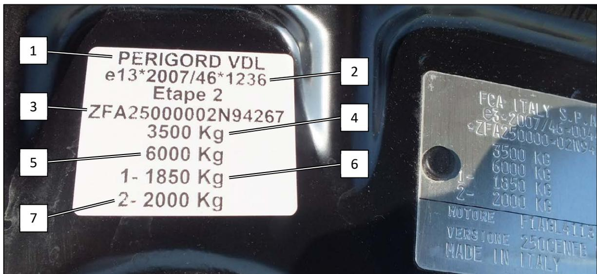
Identification plate in the engine compartment (sample illustration)
