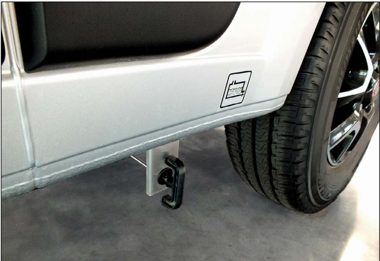
Handle for draining the waste water tank
